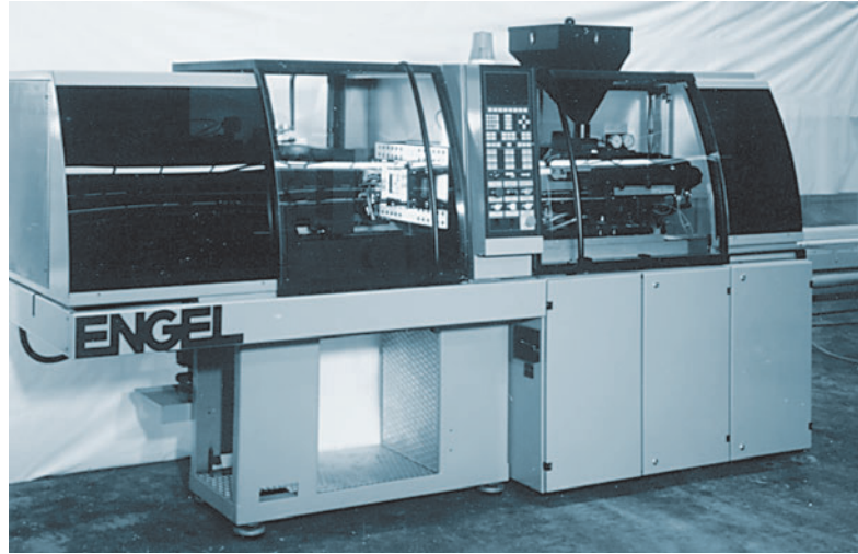
Fig. 16. Modern-day injection moulding machine (manufacturer: Engel)
