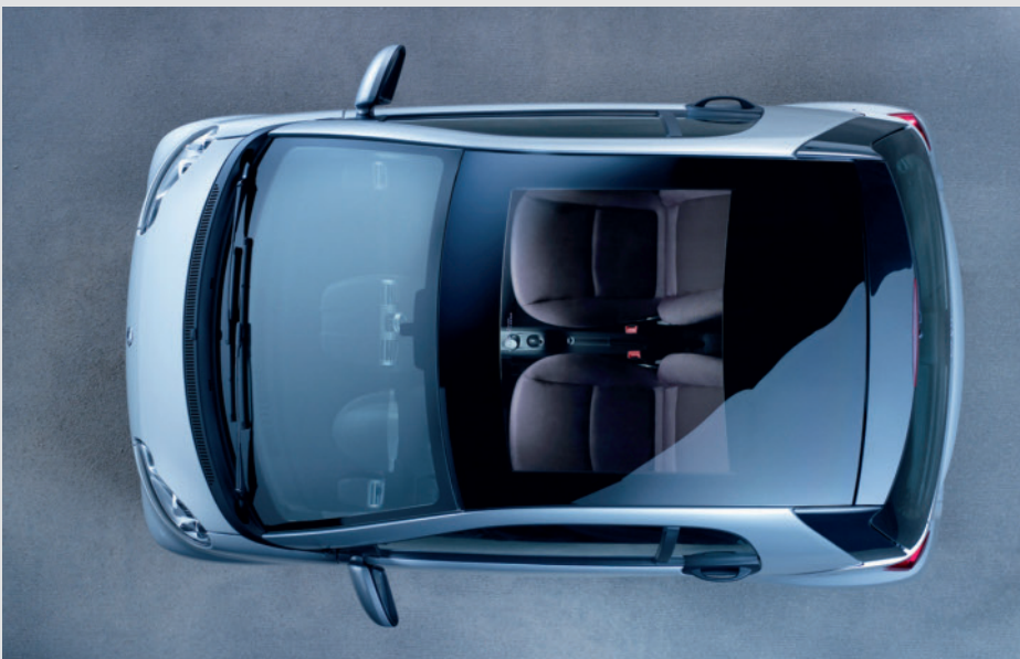
Fig. 4. Smart roof: the latest Smart car has a panoramic roof made from polycarbonate
