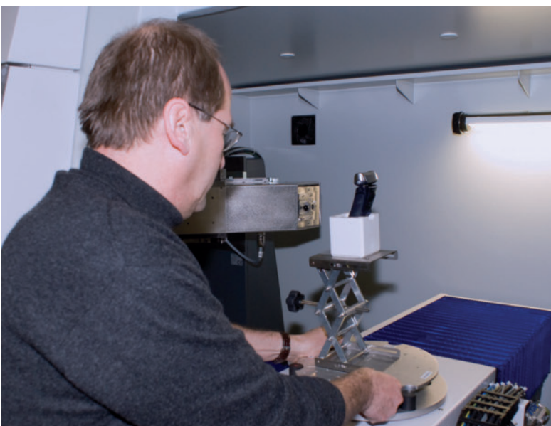
Fig. 1. The project manager prepares the test setup for a shaver: here he is adjusting the height of the electric shaver for the X-ray section
