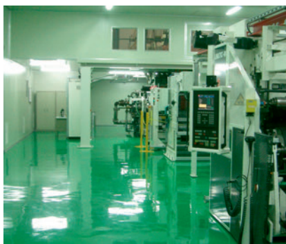
Fig. 9. Filmex cast film line in a cleanroom for production of film used to protect sensitive surfaces (photo: W&H)
