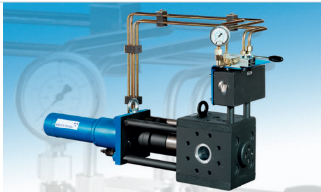
Fig. 2. Hydraulically actuated D-SWE piston screen changer (discontinuous) (photo: Kreyenborg)
