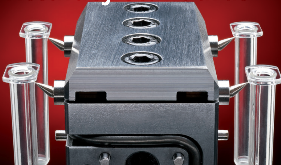
HPS III-MH linear hot-runner nozzle with moldings (figs.: Ewikon)
