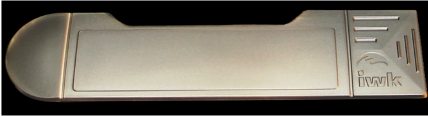
While backmolding metal sheets, the metal sheet, as the binding element, is activated by high-performance heating prior to injection (photo: IWK)
