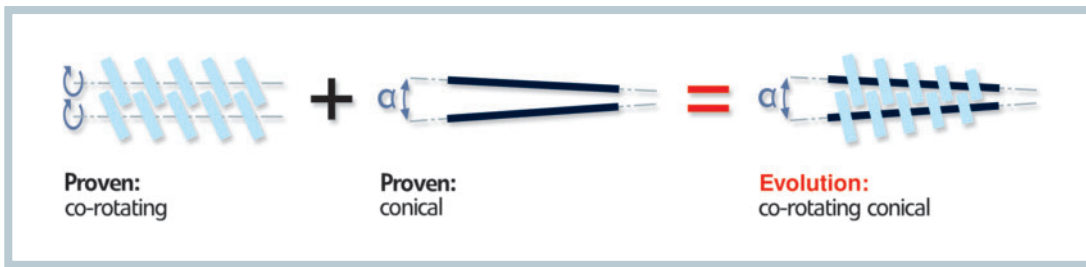
Fig. 1. The developed extruder combines two proven designs, the co-rotator and conical, into a new system
