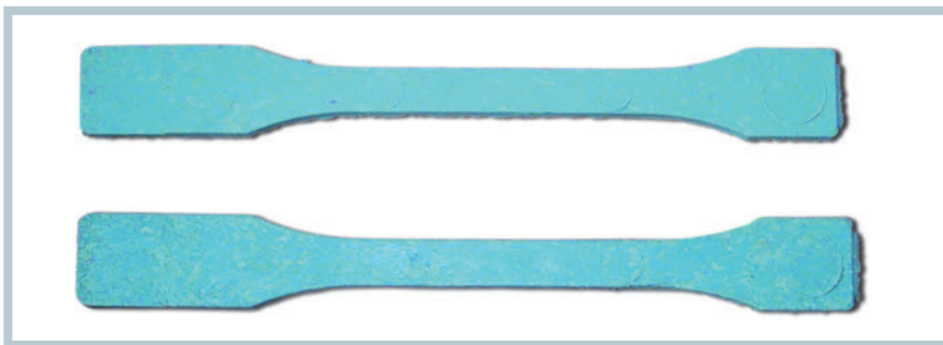
Fig. 4. Tensile specimens made from paper/plastic composite are compared for their homogeneity: NCT extruder (top) and counter-rotator (bottom)
