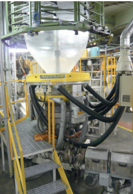
Fig. 7. Retrofitting a double cooling ring (photo: Plast-Control)
