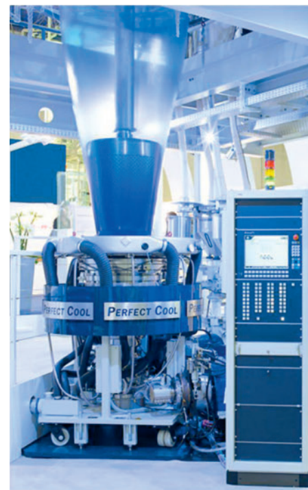
Fig. 6. ECP interior cooling system (photo: Kiefel)
