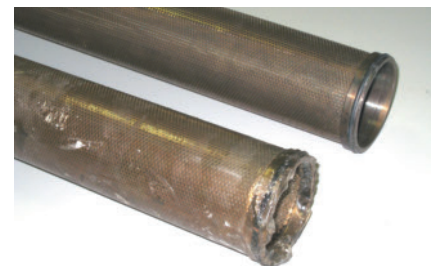
Fig. 2 . For DIC Performance Resins, pyrolytic cleaning is the most economical way of eliminating contaminants and resin residue from all kinds of installation components because it is non-destructive: shown here are pipe filters: contaminated filter (foreground), after pyrolysis (background) (photo: DIC Performance Resins)
