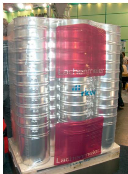
Fig. 3. One of the most important applications in terms of volume of elastic films is the stretch hood for securing pallets
