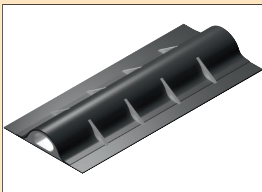
Hybrid high-performance composites integrating hollow profiles can be created by forming and combining organic sheets (photos: Bond Laminates GmbH /LKT, Erlangen-Nuremberg University)
