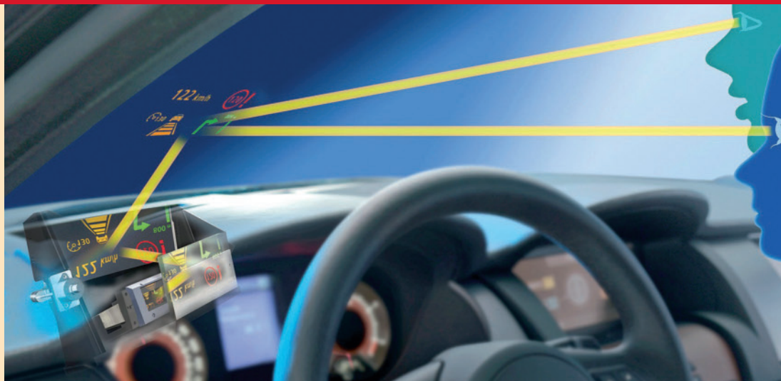
Head-up display: plastic mirrors project information into the cockpit
