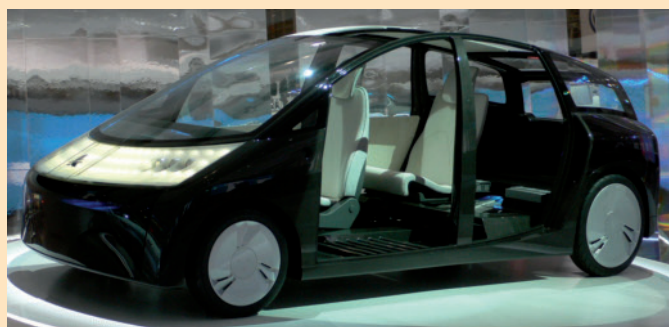
The ultra-lightweight concept vehicle 1/X with body structures made from carbon fiber-reinforced plastics weighs only 420 kg (photo: Toyota)
