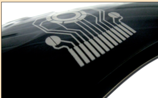
The electronics printed on the film are applied to an injection molded part and overmolded with a transparent, scratch-resistant cover layer of reactive polyurethane by means of the Clearmelt process (photo: plastic electronic GmbH)
