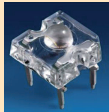
LED housing molded onto a prestamped metal carrier (left) and encapsulated LED with mold-on lens for light distribution (photos: Engel)
