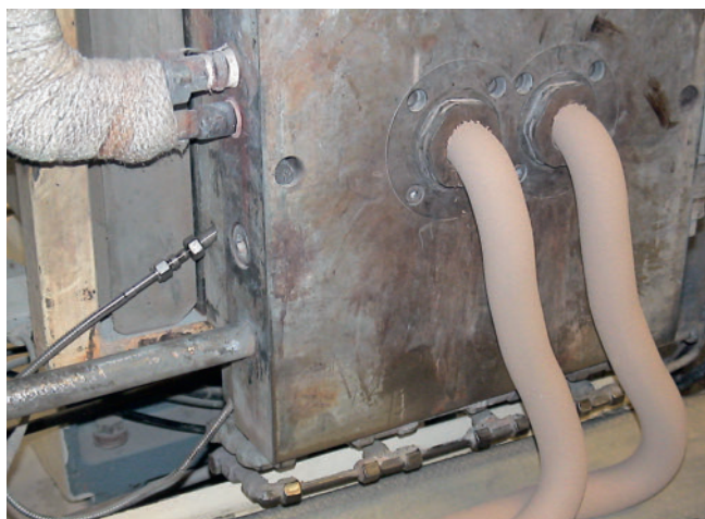
Fig. 1. The extruder probe (left) is screwed on at the side of the extruder exit opening
