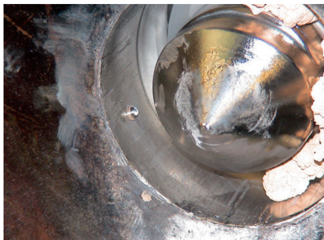
Fig. 2. The tip of the measuring probe extends into the extruder to ensure that the lens is covered with melt
