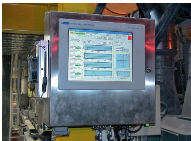
Fig. 3. The Nema 4 box with its touchscreen holds all the measuring technology
