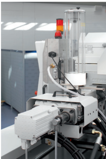
Fig. 11. Water-cooled electric drive of a metering unit
