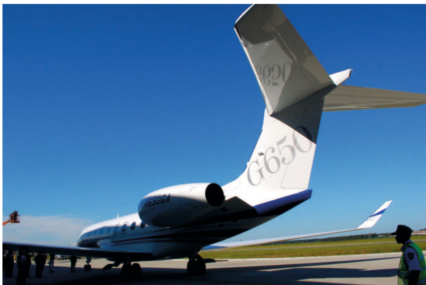
The rudder and elevators for the Gulfstream G650 were manufactured from Fortron PPS (photo: Gulfstream Aerospace Corporation)
