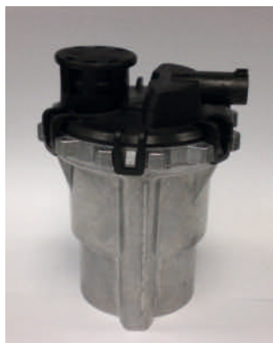
Fig. 1. The AdBlue membrane pump P800 from Thomas Magnete with a valve block made from Fortron PPS 1140L4 (photo: Thomas Magnete)
