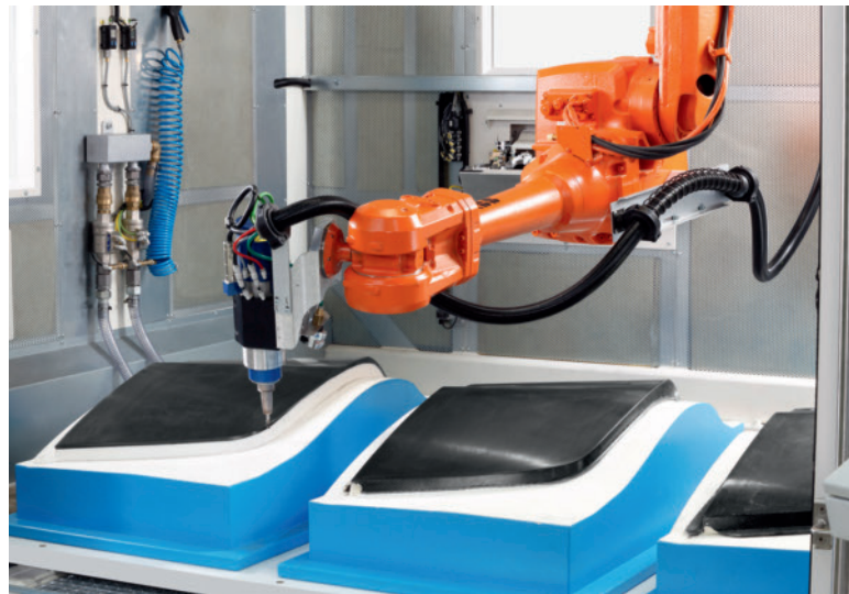
Fig. 4. The effective and production-ready machining of structural parts takes place in a milling cell
