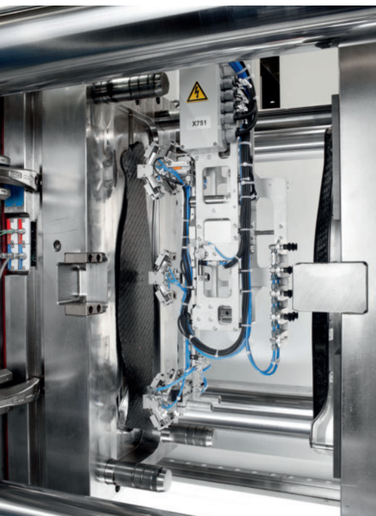
Fig. 6. Insertion of a heated organic sheet into the injection mold and removal of a pre-finished molding on the opposite side occur synchronously
