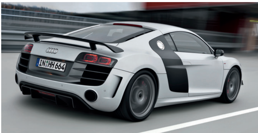
Fig. 4. The Audi R8 GT is around 100 kg lighter than the Audi R8 Coupé
