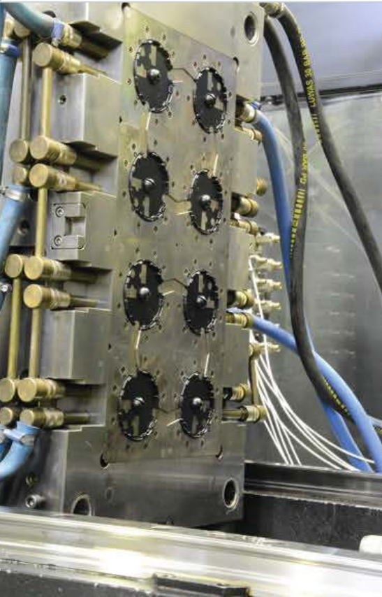
Fig. 1. Eight-cavity hot-runner mold for manufacturing base plates for adjustment motors of side mirrors. For automatic hot-runner balancing a temperature sensor is incorporated into each cavity, and a pressure sensor is additionally incorporated into one cavity for quality control
