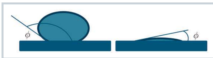
Fig. 1. Poor wetting (left) and good wetting (right) (figure: VW)
