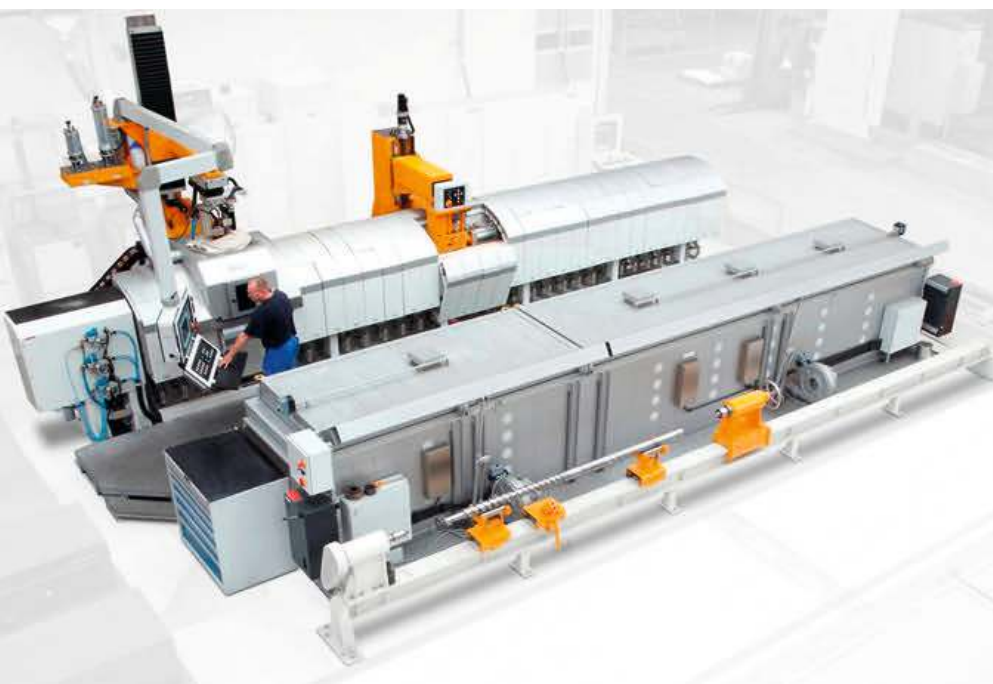
Fig. 5. Plasma-powder overlay welding machine
