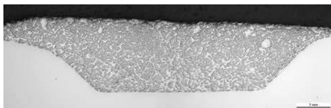
Fig. 7. Homogeneous, isotropic carbide distribution of a WC overlay weld, surface hardness approx. 58 HRC
