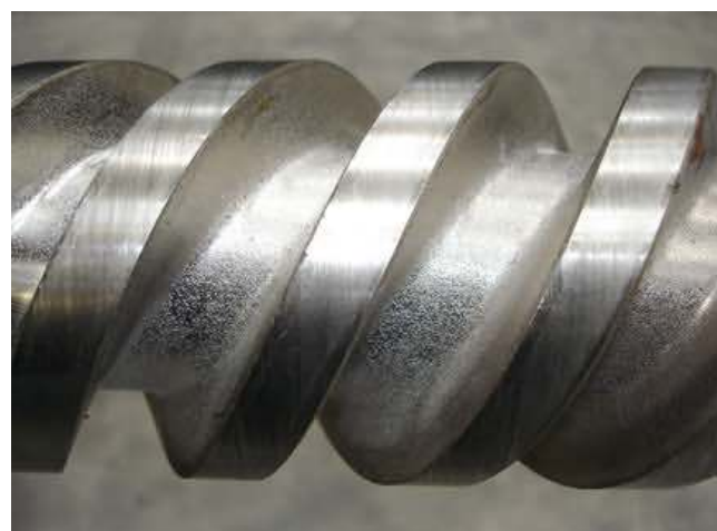
Fig. 2. Abrasive wear on twin screws
