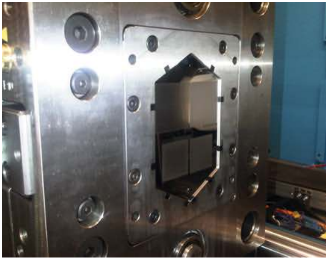
Fig. 7. Core insert with four different test zones in the CoverForm mold of an injection compression molding machine (photo: Evonik)
