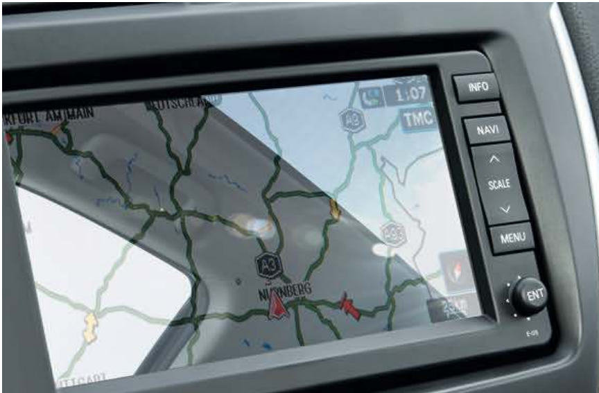
Fig. 1. Non-anti-glare surfaces on automotive dashboard instrument displays reflect the light and interfere with vision while driving
