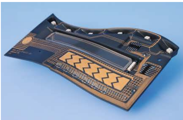
Fig. 1. In the cylinder printing machine, the MyWave-3D is decorated in a total of seven screen printing runs
