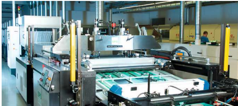
Fig. 1. In the cylinder printing machine, the MyWave-3D is decorated in a total of seven screen printing runs
