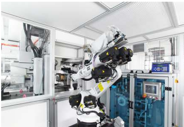
The final packaged product is produced in one step: a six-axis robot removes the drill, molded on an electrical Allrounder 370 A and transports it to the packaging unit (right in the left picture, with the blue glazing)
