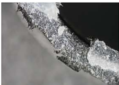
Fig. 1. Material that sticks on indicates that this is a cohesive fracture as desired
