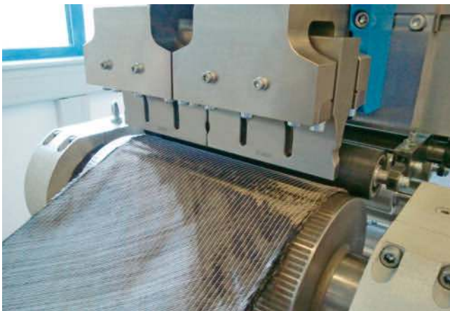
Fig. 4. Lab setup with stationary sonotrodes: welding carbon fiber mats with ultrasonic vibrations
