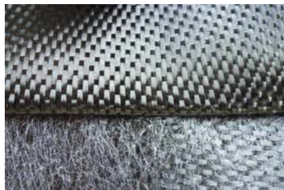
Fig. 1. Thermoplastic adhesive fabric between layers of carbon (figures: Herrmann Ultraschall)
