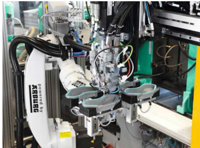
Fig. 3. The PU gasket foam is applied directly to the still-hot plastic parts after injection molding (photo: Arburg)
