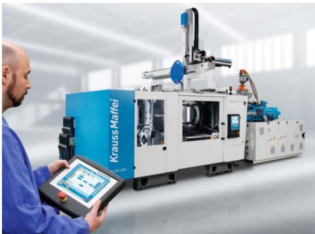
Fig. 1. The robot and machine can be programmed and operated using the machine control and robot-handheld (photo: KraussMaffei)
