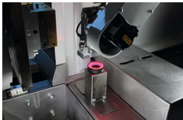
Fig. 14. The optical checking of the part quality – here with an integrated camera with LED illumination – is already a widespread standard (photo: Wittmann)
