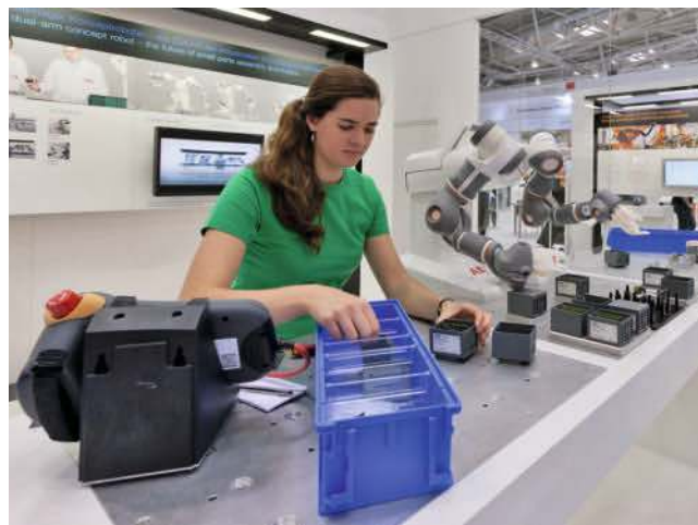
Fig. 4. The two-arm draft robot with flexible grippers and camera-based parts recognition is being developed for assembly environments that require cooperation with humans (photo: ABB)
