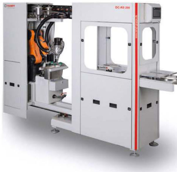
Fig. 8. With the Kuka Agilus, this compact metering cell, shown open here, uses a special six-axis robot (photo: Rampf Dosiertechnik)
