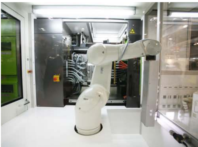
Fig. 6. Six-axis robots in cleanroom design is suitable for sensitive applications, such as here in medical technology (photo: Stäubli)
