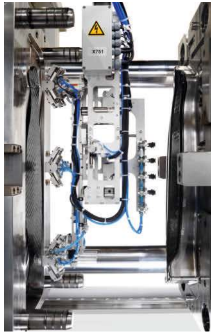
Fig. 13. The challenge during insertion of semi-finished products comprising an endless fiber-reinforced textile impregnated with a polymer matrix into the mold is to handle the prepared, heated organic sheet with a needle gripper (photo: KraussMaffei)
