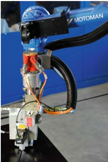
Fig. 5. A process filed for a patent in 2011 simplifies bonding and sealing applications. Parts no longer have to be produced with accurate joints and an accurate fit, because a new system comprising six-axis robots, metering technology and 2-D laser sensor reliably seals different gap sizes from 2 to 7 mm
