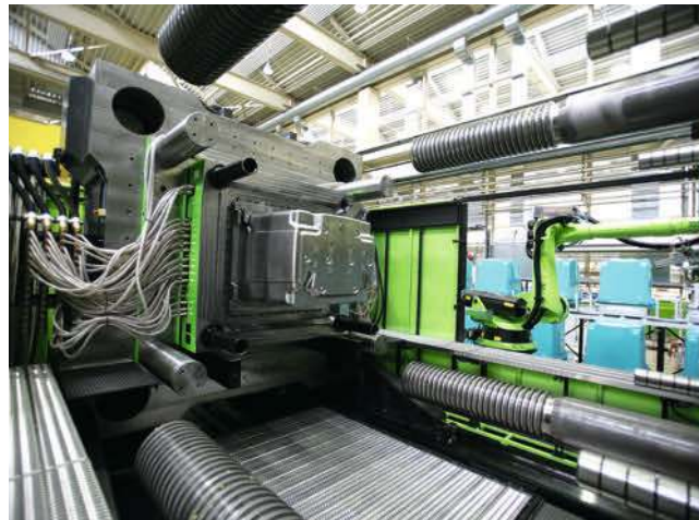
Fig. 7. The larger the machine, the higher the degree of automation with industrial robots. Here, a Kuka robot on the seventh drive axis serves a 55,000 kN injection molding machine producing the trash containers
