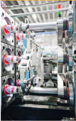
Fig. 9. Production of yogurt cups by the in-mold labeling process with simultaneous removal of parts and insertion of labels by a double gripper (photo: Sumitomo (SHI) Demag)
