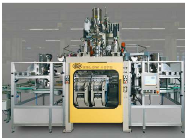
Fig. 1. The EBlow 407 D with a all-electric drive is a twin-station blow molding system for hollow articles with a volume up to 10 liter (photo: Bekum Maschinenfabriken)
