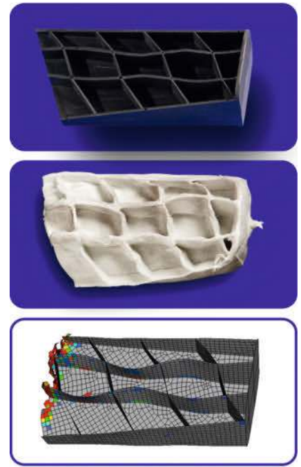
Fig. 3. Long glass fiber reinforced polymers form a three dimensional glass fiber network during injection molding (center of picture), which gives the component its exceptional mechanical performance for instance as a bodywork crash absorber. The behavior of such demanding components can now also be calculated and predicted via computer simulations
