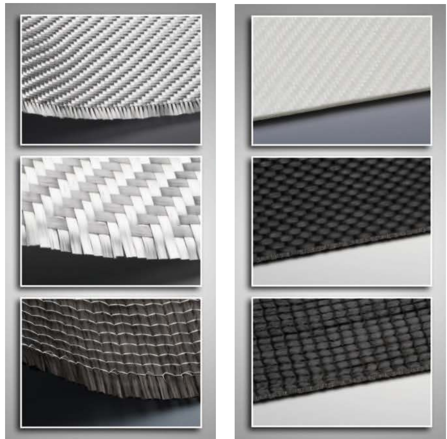
Fig. 9. Various glass and carbon fiber textile structures based on wovens and non-wovens (left); various RTM fiber composite laminates based on polyamide, polyurethane and epoxy resin (right)
