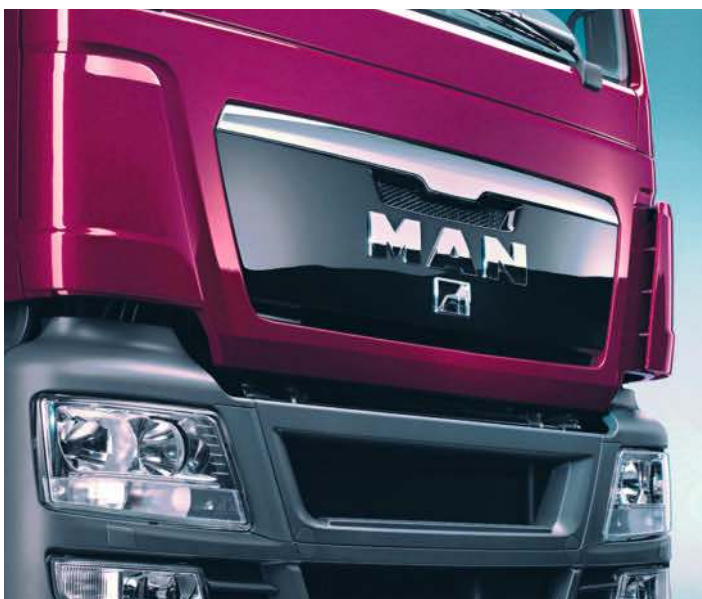
Fig. 4. Long fiber reinforced polyurethane is already being used for the MAN radiator grills (photo: MAN-Truck)
