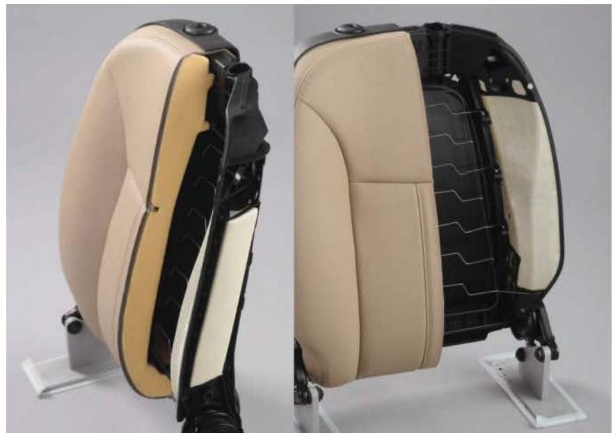
Fig. 6. The prototype SUSCO 1.5 seat from Faurecia was developed jointly with BASF and uses continuous fiber thermoplastic tapes in the seat back (white in the picture) which in a second process are overmolded with a special polyamide (black seat back parts). The replacement of the existing metal structure in the seat backs with a single piece polymer component reduces the weight of the back by about 20 %
