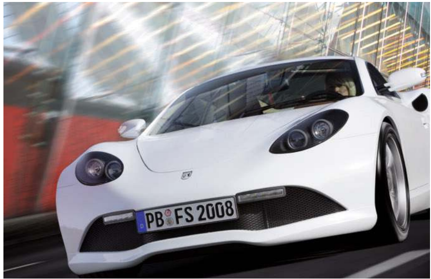
Fig. 1. The bodywork of the Artega GT, a low volume sports car made in Delbrück, Germany, consists mainly of polyurethane reinforced with short mineral and carbon fibers
