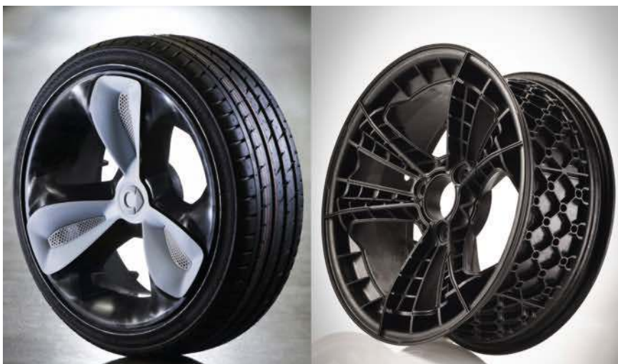
Fig. 2. The new smart forvision concept car presented at the IAA 2011 was equipped with the world's first thermoplastic wheels that have the potential to be mass produced. They are made from long glass fiber reinforced polyamide and with a weight of 6 kg they are some 30 % lighter than mass produced aluminum wheels reducing the overall weight of the vehicle by 12 kg
