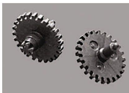
Precise metering is essential for the production of microparts. The barely 2 mm-diameter gear wheel weighs only 1 mg
