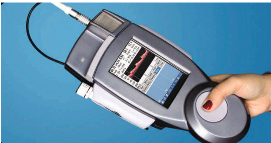
Fig. 2. For the housing of this portable device from Multigon Industries, which is used to detect unseen traumatic brain injuries on site, a plastic compound incorporating stainless steel fibers provides a cost-saving alternative to metal-oversprayed plastic, while delivering equivalent electromagnetic shielding performance
