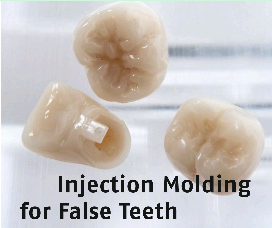
Teeth manufactured in the injection molding process, scarcely distinguishable from “real” teeth. An adjusting pin at the tooth root serves to fix the artificial teeth (figs: Günther)
