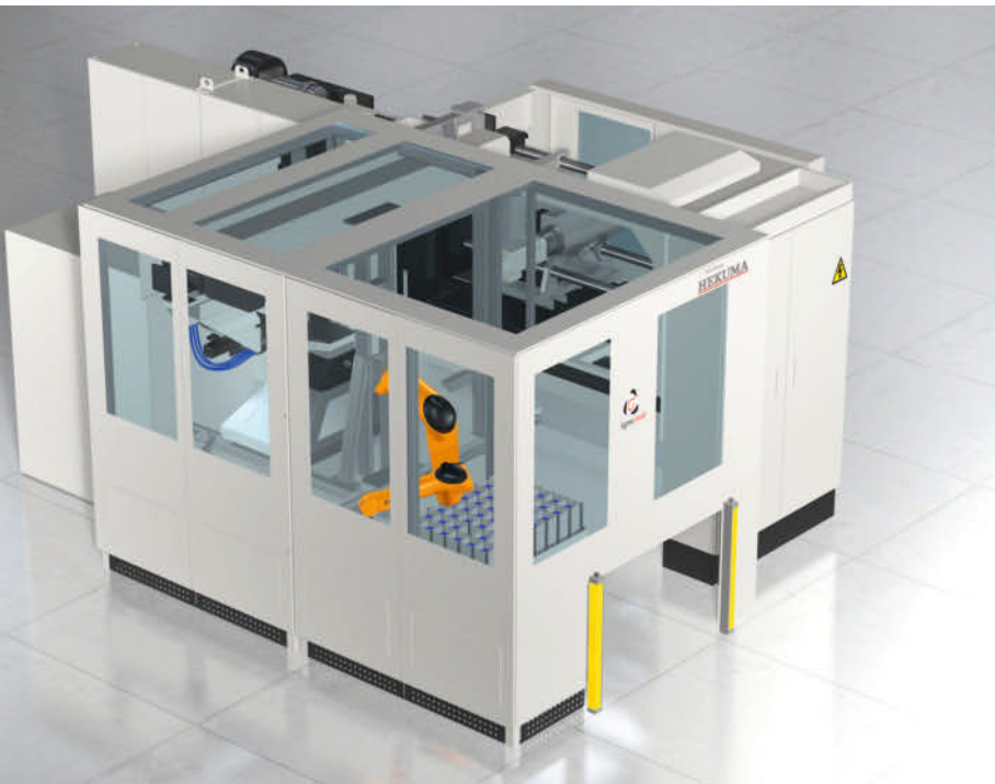
The molded parts emerging from the clean room cell are sorted into individual containers for further processing or shipping (photos: Hekuma)
