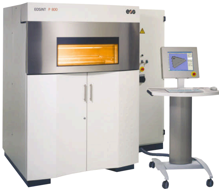
Fig. 1. Eosint P 800 laser-sintering system used to manufacture high-temperature PEEK cranial implant prototypes for Custom IMD research project
