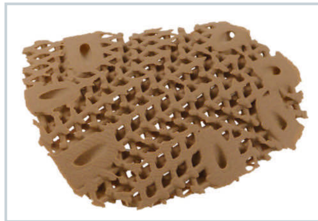
Fig. 2. An early design showing the PEEK scaffold structure that was manufactured in one piece by laser-sintering. While it was a good fit, it offered little scope for osseointegration
