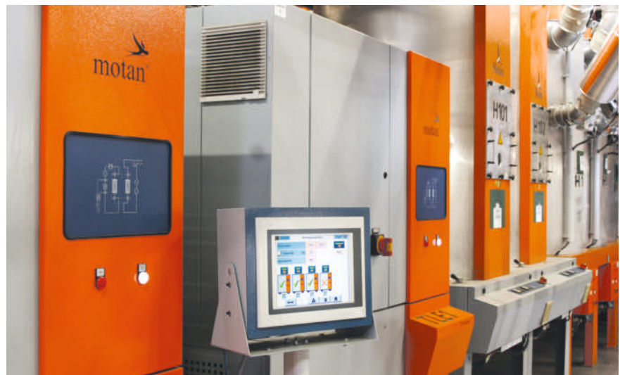
The control and operation of the system can take place both locally on the individual units and centralized via a visualization system
