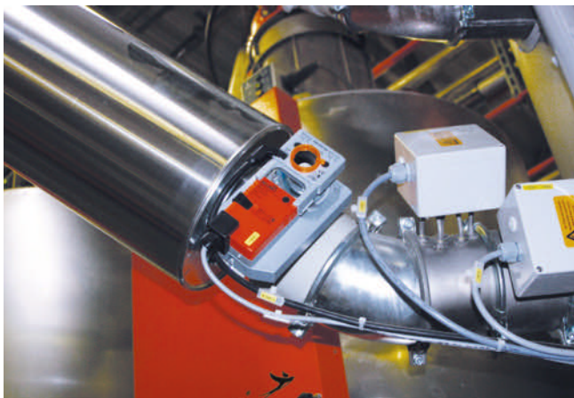
If the control system recognizes that the material in the bin is completely dry, the air flap reduces the throughflow
