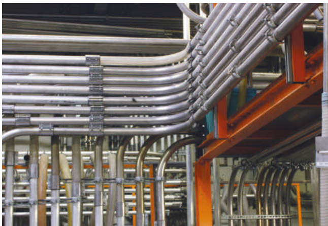
The centralized conveyor feeds 150 conveying points
