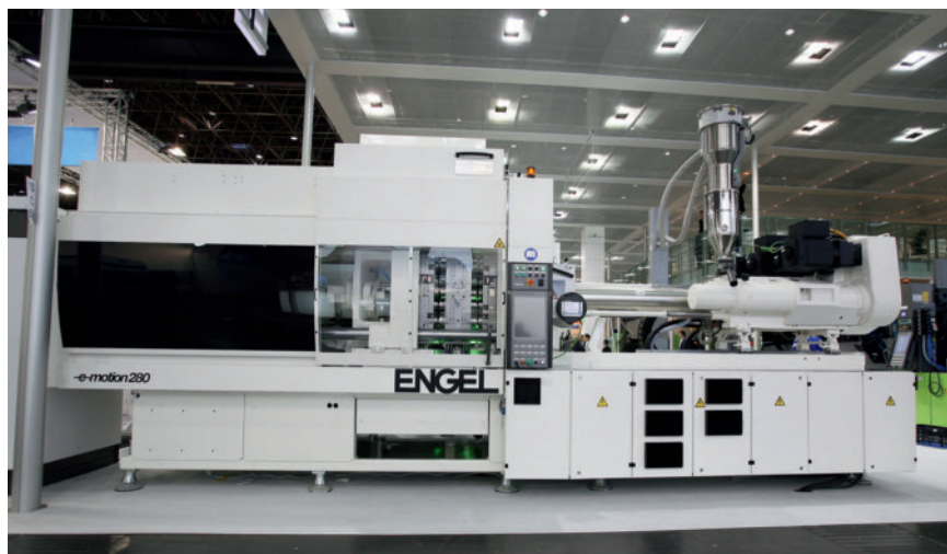
Fig. 4. The all-electric injection molding machine satisfies the requirements for use in a cleanroom. At the trade fair, polystyrene Petri dishes (right) were molded using an 8+8-cavity mold (supplier: Plastisud, Castelnaudary, France) at a cycle time of 3.6 s (photos: Engel)
