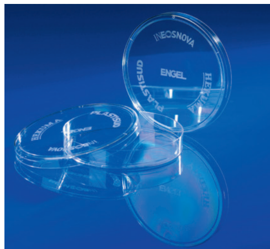
Fig. 4. The all-electric injection molding machine satisfies the requirements for use in a cleanroom. At the trade fair, polystyrene Petri dishes (right) were molded using an 8+8-cavity mold (supplier: Plastisud, Castelnaudary, France) at a cycle time of 3.6 s (photos: Engel)
