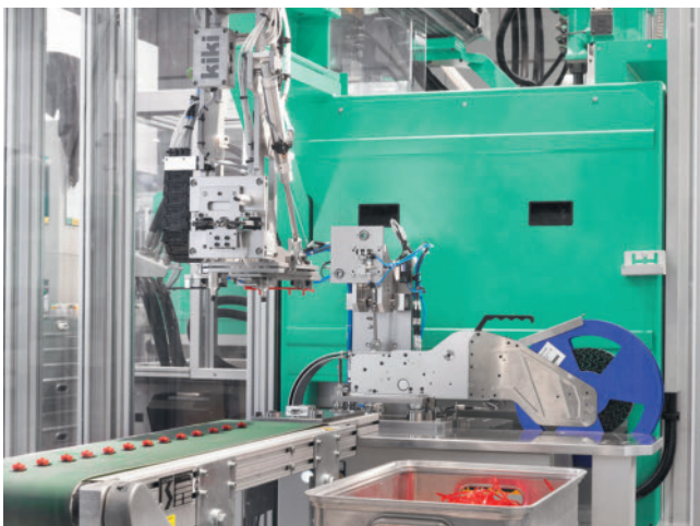
Fig. 1. The linear robot loads the contact pins precisely, transfers the pre-shots and assembles three individual components to yield the finished part – see conveyor belt (photo: Arburg)
