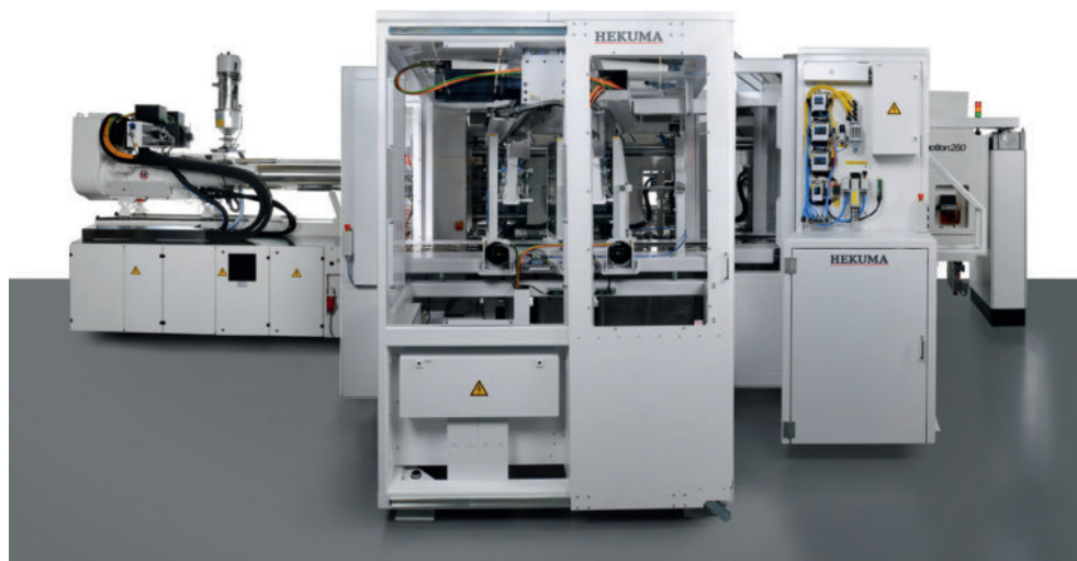
Fig. 4. The production cell can be configured to manufacture Petri dishes under cleanroom conditions, for instance (photo: Hekuma)
