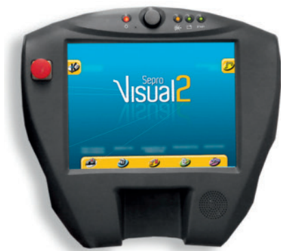
Fig. 6. The Visual 2 CNC controls permit remote access for service by specialists (photo: Sepro)
