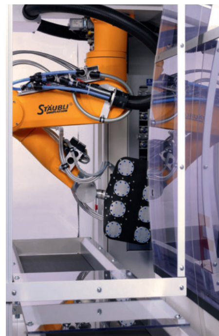
Fig. 7. Arm length, payload and cleanroom version of the six-axis robot can be matched to the requirements of the cell (photo: Stäubli)
