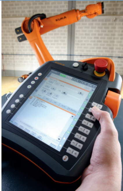
Fig. 8. The KR C4 controls with touchpad integrate a wide variety of functions yet remain easy to operate (photo: Kuka)
