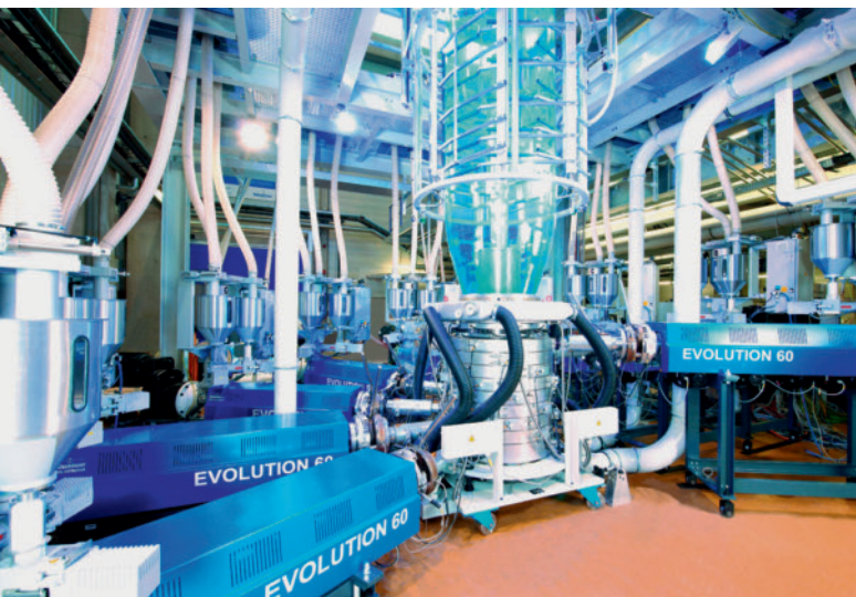
Fig. 2. Nine-layer blow head of the new generation of Evolution lines
