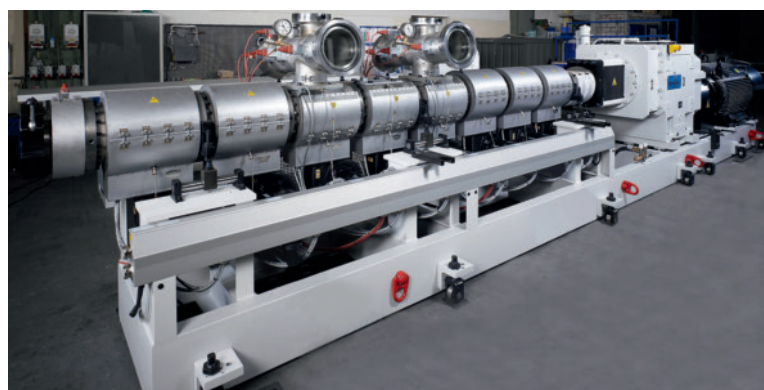
Fig. 5. Reitruder RZE with concurrent twin-screws and degassing unit for the direct processing of recycled PET (photo: Reifenhäuser)
