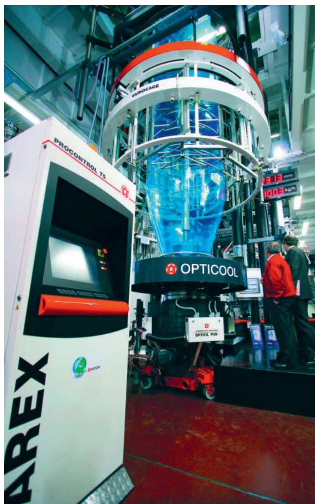
Fig. 1. With its new cooling ring, the new VAREX 5-layer blown-film line configured for polyolefins achieves outputs in excess of 1,000 kg/h
