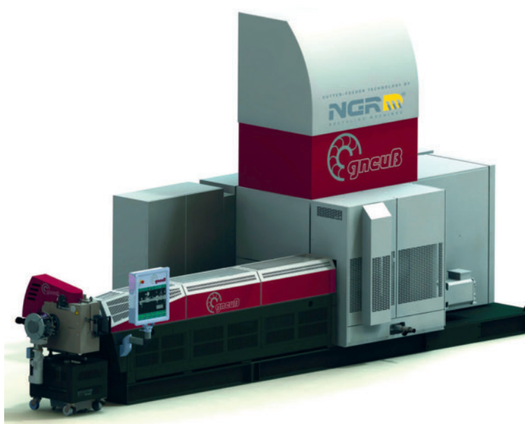
Fig. 6. Complete line with cutter-feeder unit for the direct recycling of PET fibers or film wastes (photo: Gneuss)
