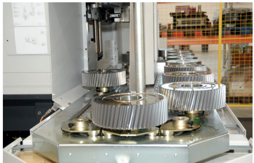
The new fully automated CNC cutting machines for mass producing gears is fast, flexible and integrated with an automatic robot system
