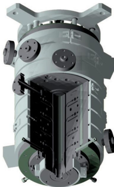
Fig. 10. Seven-layer blown film die for biaxially-stretched films (double/triple bubble)
