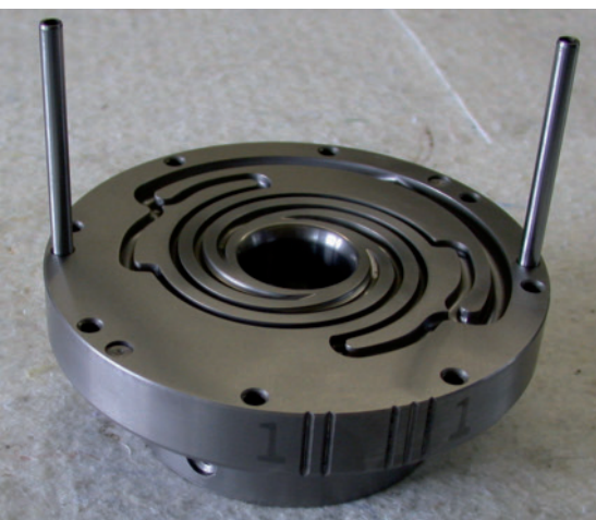
Fig. 7. Circular distributor plate and single-layer die for micro-hoses
