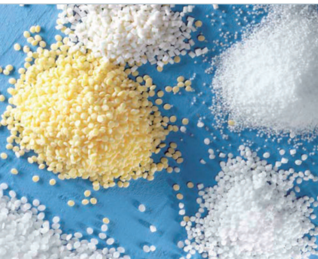
Endothermal (white) and exothermal (yellow) masterbatches of blowing agents
