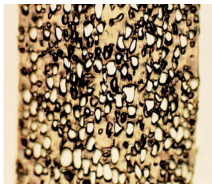
Fig. 3. Microscopic presentation of the foam structure in a PET mono-film (thin cut, amplification 1:100, density 0.87 g/cm 3 )
