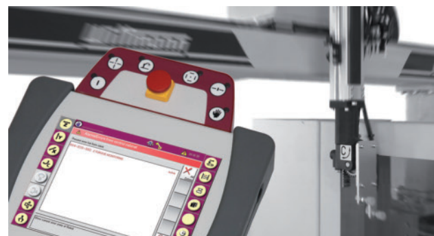
Fig. 2. The new R8 control generation offers active collision protection (photo: Wittmann)
