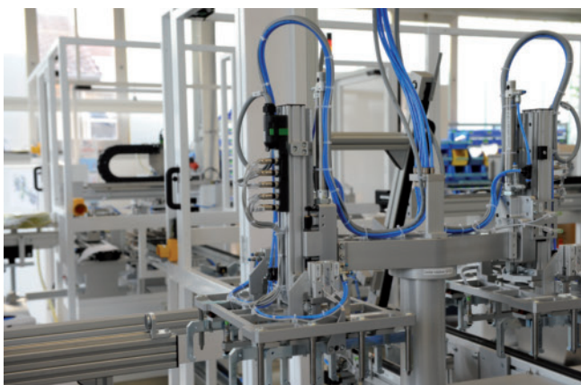
Fig. 11. Modular handling systems permit customized alignments
