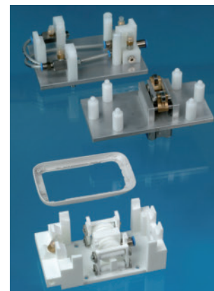
Fig. 6. Laser sintered handling components are aligned to individual jobs (photo: ASS)
