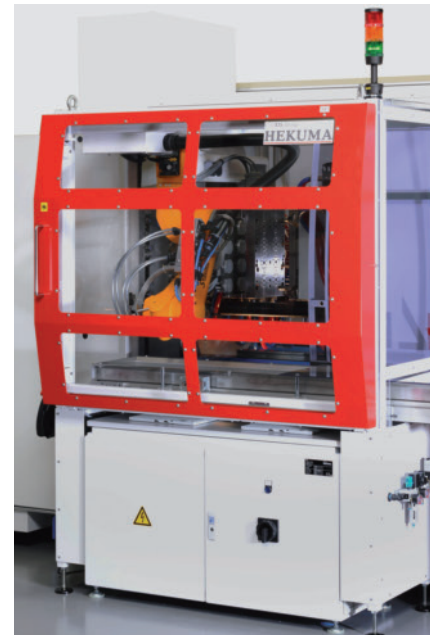
Fig. 9. The HekuCell as a standard module for automating part removal on small and medium-sized injection molding machines (photo: Hekuma)
