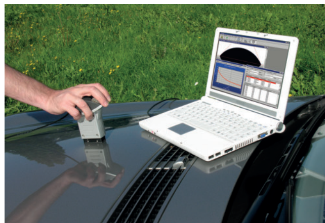
Fig. 1. The MobileDrop permits contact angle measurement on inclined surfaces or very large samples (photo: Krüss)
