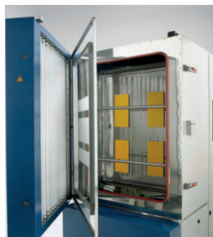
Fig. 5. The UV200 global UV test instrument performs weathering tests based on acid rain (photo: Weiss)
