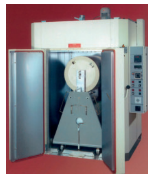
Fig. 7. The tilting rotating drums with traversable frame keep small plastic parts in motion during tempering (photo: Vötsch)
