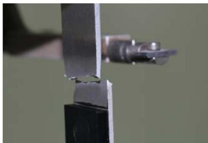
**Fig. 1.** Metal tears, hybrid holds: The high adhesion between metal and plastic leads to a fracture in the aluminum (© Akro-Plastic)
