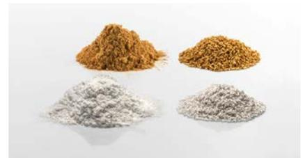
**Fig. 5.** Dust-free handling of Mastersafe Symic pearlescent pigments is assured due to their pellet form (© Eckart)
