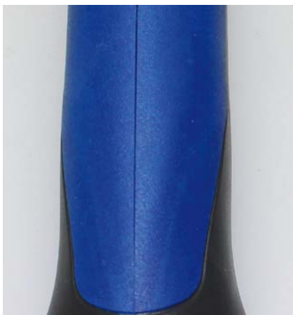
Fig. 6. Compared to the standard 2C process, the mixing nozzle eliminates color streaking (left) in the soft component (© Promix)
