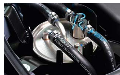
EVM rubber Levapren PXL for hoses and cable sheathings (© Arlanxeo)
