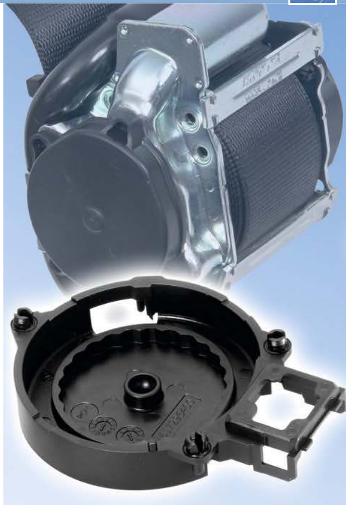
Autoliv produces these bearing plates for seat belt retractors from a low-emission and impact-modified polyacetal homopolymer from DuPont. This combines the demand for high-impact resistance with additional noise-damping properties (figure: DuPont)
