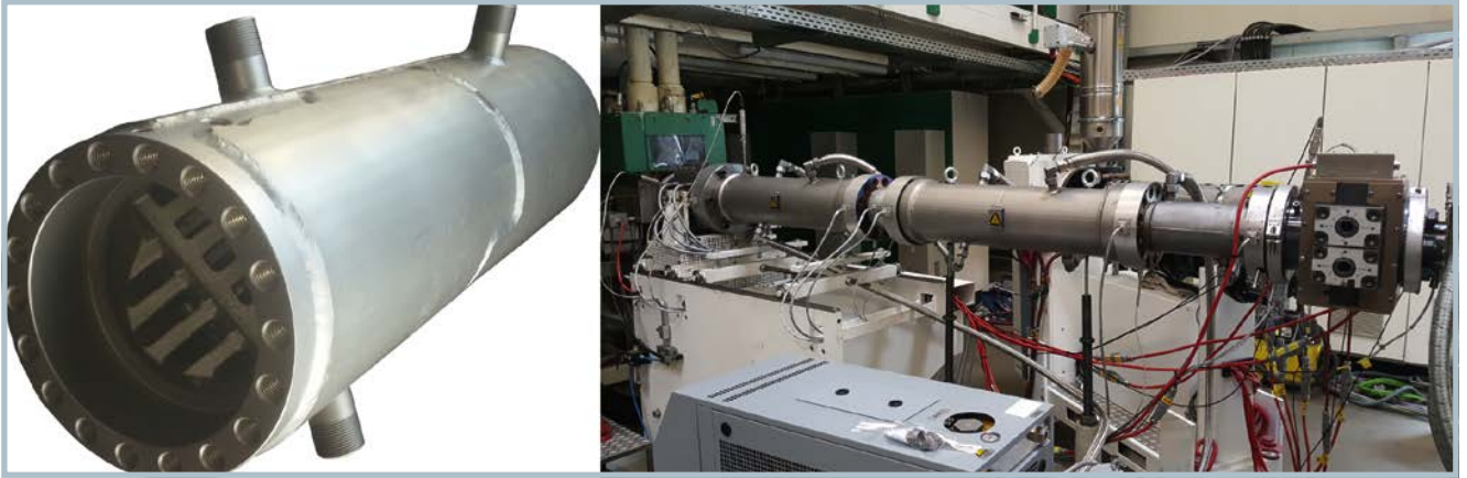
Fig. 3. Hollow channels do the trick: the P1 cooling mixer cools the melt during mixing (© Promix)
