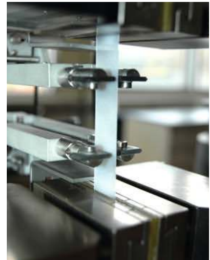
Fig. 3. Mechanical testing of the plasma treated films under tensile loading
