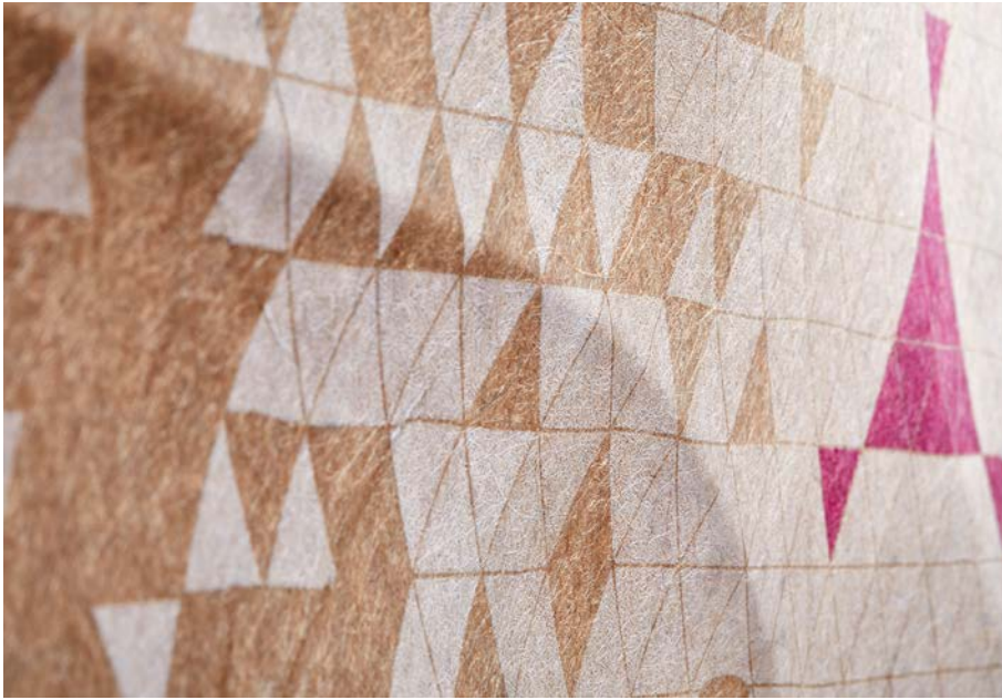
Fig. 2. The natural materials are laminated with a protective film to ensure that the surfaces meet the demands made on them. The challenge in this process is the forming of all the materials at up to 200°C (© YFAI)
