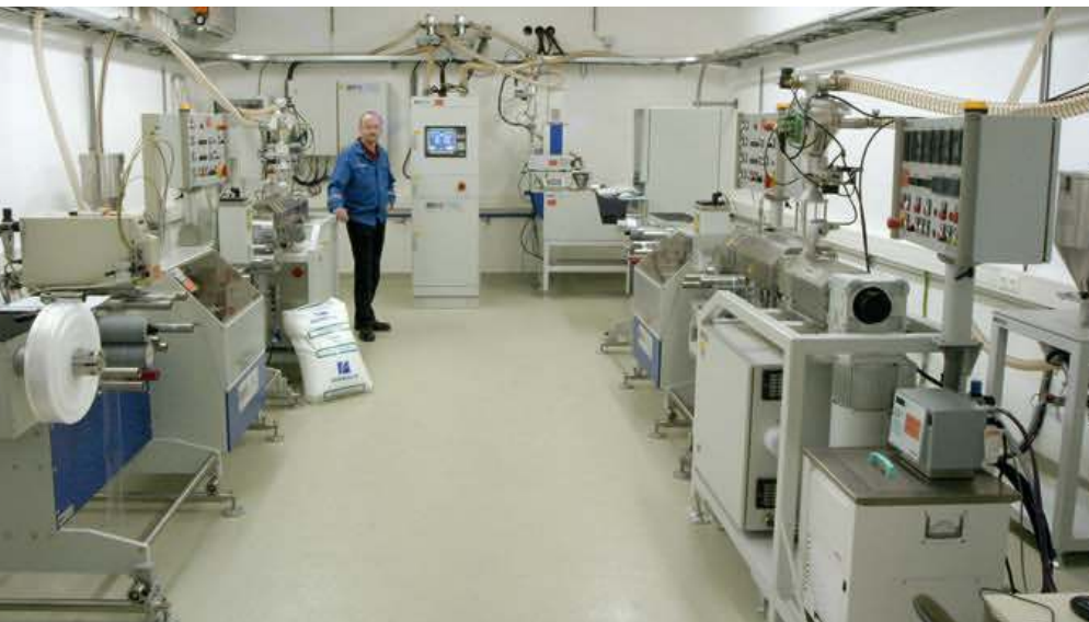
Fig. 3. Online “Closed Loop” measurement cell for two LDPE lines
