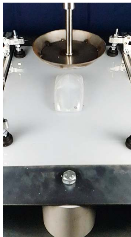
Fig. 8. Set-up of a drop test to determine the mechanical stability when using 1% Iriodin 6163 Way or 1% aluminum pigment in PP
